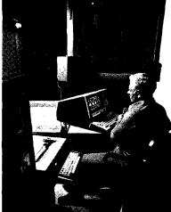
Two men can handle the job. even during peak traffic. The HP minicomputer handles all truck logging functions and automatically calculates and verifies correct load weights. Most trucks can be cleared in a little over twenty seconds. Hard copy summaries of the day's activity are available at the touch of a button.
